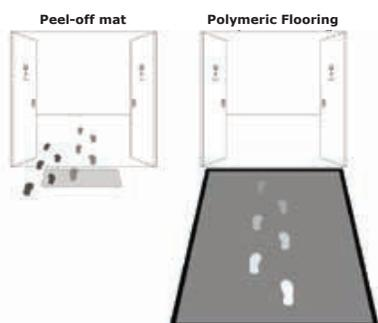
Figure 2. The overall efficiency of contamination control is dependent on the effective area of the control surface.
